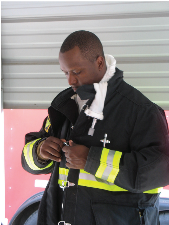
Figure 4. Fire fighter wearing a PAH sampler and respirable dust cyclone with fabricated aluminum grit pot wrapped in Nomex material. Photo by NIOSH.
