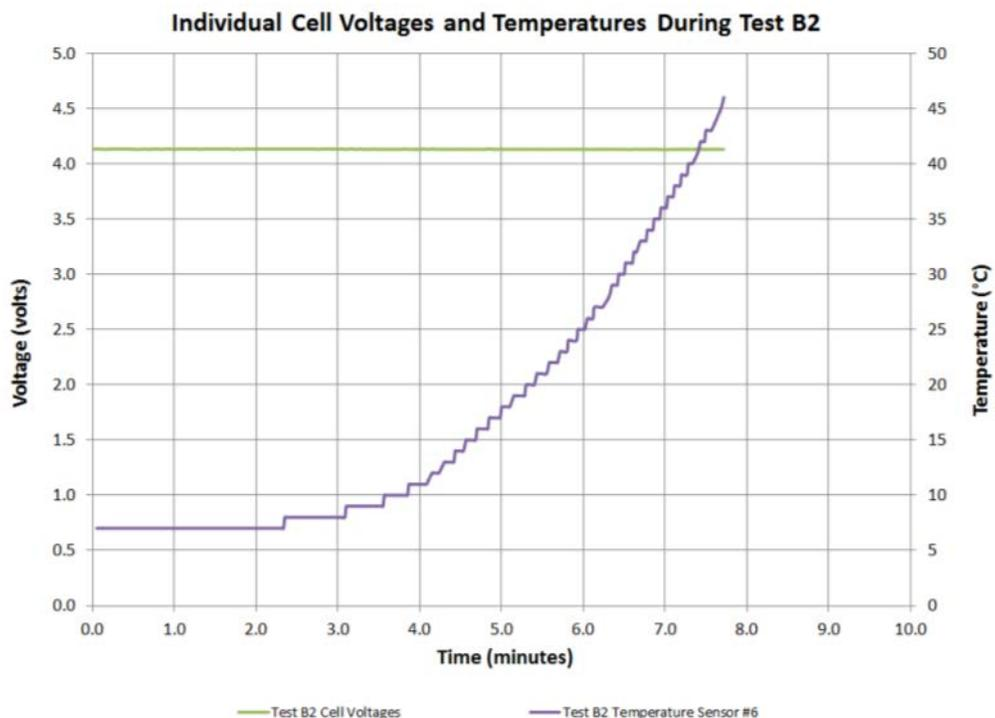
Figure 84 Internal cell voltages and temperatures during Test B2
