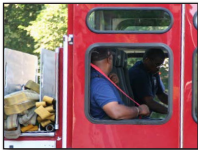
Figure 5.13 – High-visibility seatbelts are now required in NFPA standards. (Photo/Mike Wieder)
