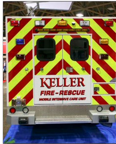
Figure 4.26 – NFPA 1917 requires reflective markings on new ambulance. (Photo/Mike Wieder)
