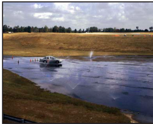
Figure 3.16 – Skid pads provide realistic wet driving surface training. (Photo/Mike Wieder)
