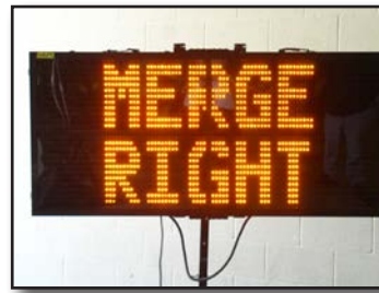
Figure 6.3 – Changeable message signs give specific directions to approaching motorists. (Photo/Ron Moore, Plano, Texas)
