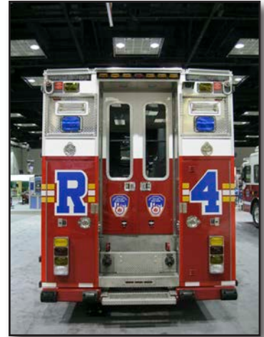
Figure 4.14 – Blue warning lights may be used on a variety of emergency vehicles. (Photo/Mike Wieder)
