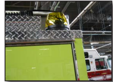
Figure 8.29 – Some agencies revert to all amber lighting once parked on the emergency scene. (Photo/Mike Wieder)
