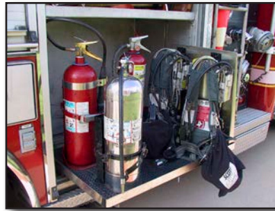
Figure 4.7 — SCBAs should be mounted in exterior compartments. (Photo/Mike Wieder)
