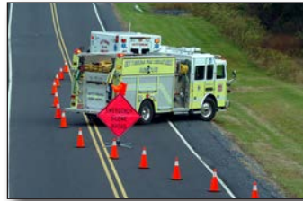
Figure 7.16 – Place the first blocking vehicle about 50 feet behind the work area. (Photo/Bob Esposito, Pennsburg, Pennsylvania)
