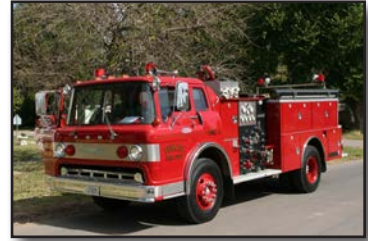
Figure 7.11 – Older fire apparatus are not equipped with ABS. (Photo/Perkins, Oklahoma Fire Department)
