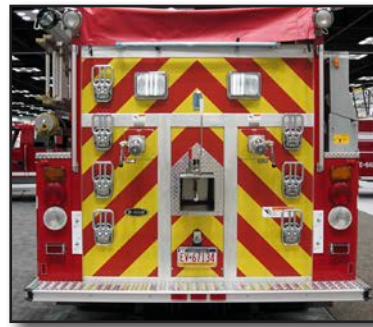
Figure 4.24 – New fire apparatus are required to have reflective markings on various parts of the vehicle. (Photo/Mike Wieder)
