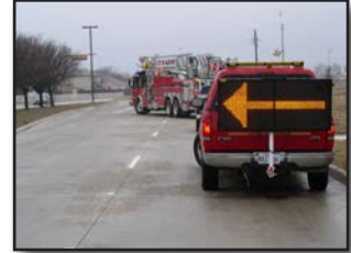
Figures 6.5a and 6.5b – A vehicle-mounted changeable message sign. (Photo/Ron Moore, Plano, Texas)
