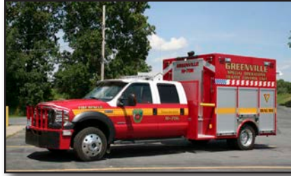
Figure 7.33 – Some fire departments operate fire police units that have vehicles designed specifically for traffic management functions. (Photo/Ron Jeffers, Union City, New Jersey)
