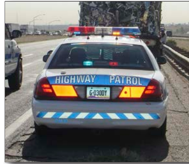
Figure 4.25 – Police vehicles may be equipped with reflective markings.
