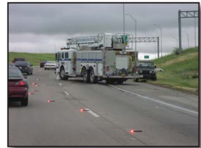
Figure 8.12 – Proper blocking positioning for a vehicle at a roadway incident scene. (Photo/Ron Moore, Plano, Texas)
