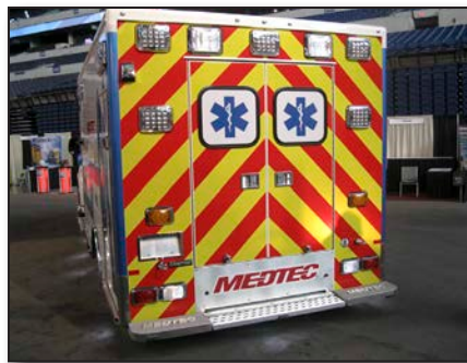
Figure 1.7 – Increased visibility techniques are used on all types of emergency vehicles. (Photo/Mike Wieder)
