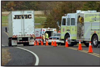
Figure 7.15 – Apparatus shall be placed to upstream side of the incident in a manner that reduces the chance of a vehicle being struck by oncoming traffic. (Photo/Bob Esposito, Pennsburg, Pennsylvania)
