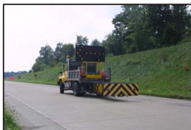
Figure 8.7 – Most transportation agencies have barrier vehicles suited for lengthy deployments.
