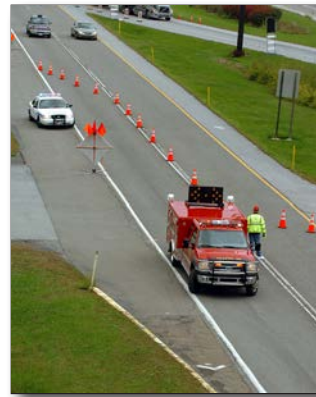
Figure 7.17 – Traffic cones assist in guiding motorists away from the incident area. (Photo/Bob Esposito, Pennsburg, Pennsylvania)
