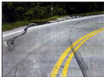
Figure 3.7 – These tire marks indicate that the vehicle's wheels left the road surface.
