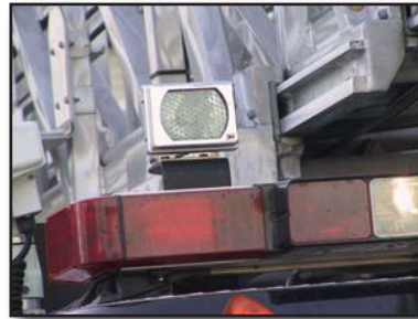
Figure 6.6 – Emergency vehicle may be equipped with emitting devices that trigger a sensor on approaching traffic signals to grant the emergency vehicle the right-of-way. (Photo/Mike Wieder)
