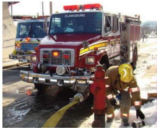
Figure 16: Connecting to the Hydrant
