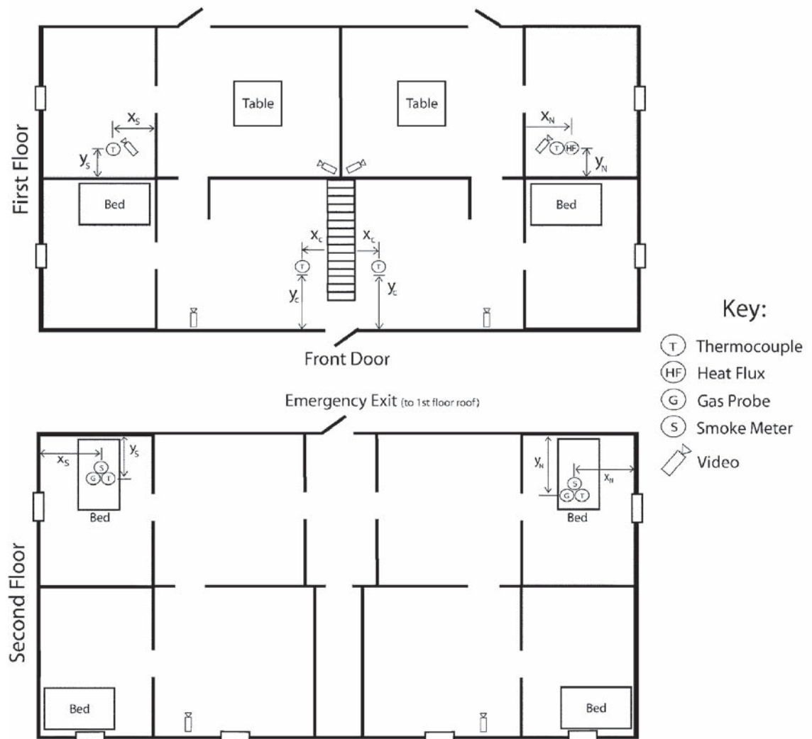
Figure 6: Instrumentation and Furniture Prop Layout
