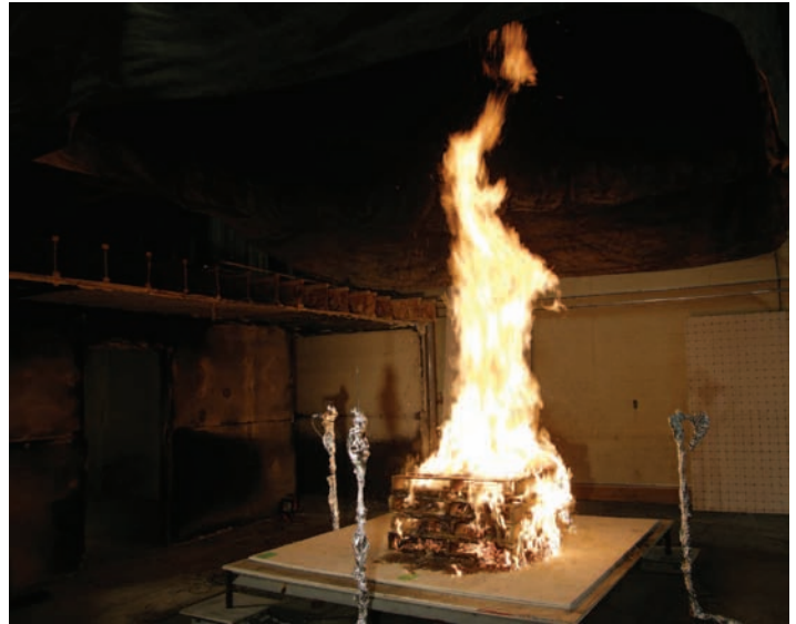
Figure 2: Test Burn of Pallets in Laboratory
