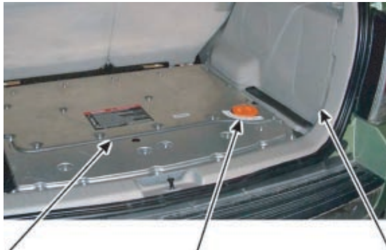
High-Voltage Battery Pack
