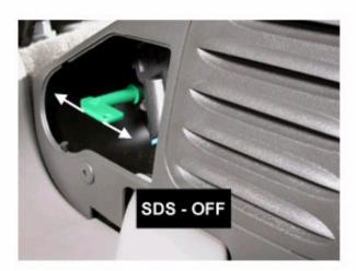
Disconnects 42 volt battery from vehicle electrical system:
