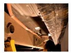
Is the 120-volt harness visible on the bottom of the vehicle? NOTE: Orange loom used only by high voltage systems.
