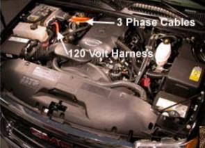
Starter/Generator Control Module (SGCM) Electrical System Connections (Continued)
