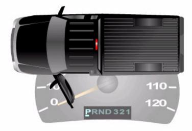
If the vehicle is in the automatic engine start-stop mode and in Park with the engine off, the engine will start if either vehicle door is opened.
