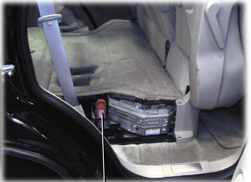
300V Hybrid Battery Manual Disconnect
