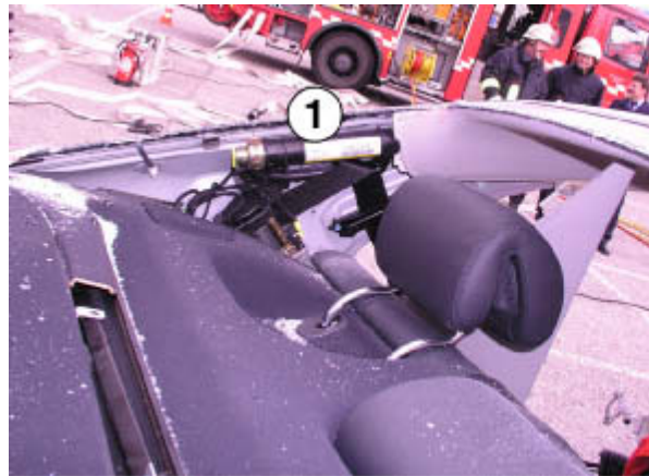
1 Compressed gas generator in the C-pillar
