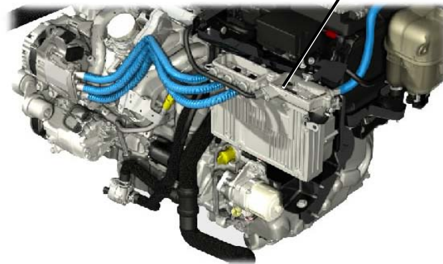
Cables from the Generator with Starter, 12v battery and 36v battery enter the top of the Generator Control Module (cover removed for clarity)
