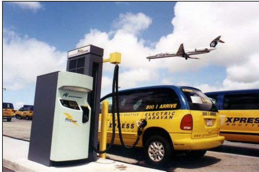
Figure 3-17: EV Taxis at a Charging Station (Photo courtesy of NREL Photographic Information Exchange)
