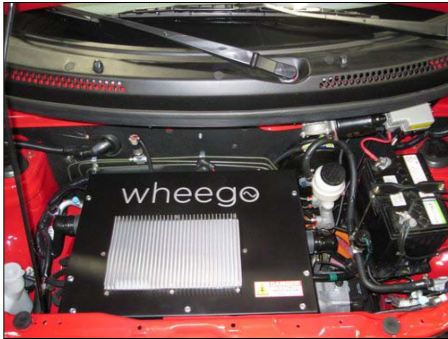
Figure 5-5: NEV High Voltage and Low Voltage Battery Modules (Photo courtesy of NREL Photographic Information Exchange)
