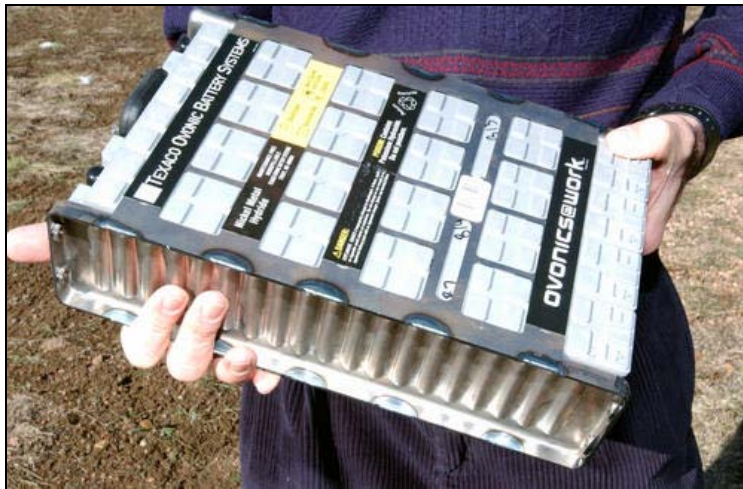
Figure 2-5: NiMH Liquid Cooled EV Battery Module (Photo courtesy of NREL Photographic Information Exchange)
