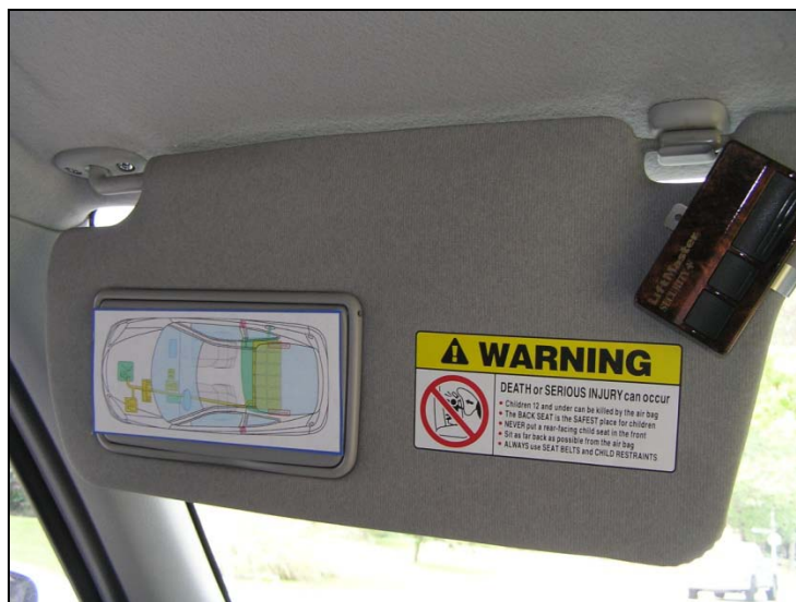
Figure 3-10: Example of VSDS Concept 96 (on left, with standard visor warning label in center and typical garage door opener on right) (Photo courtesy of Ron Moore)
