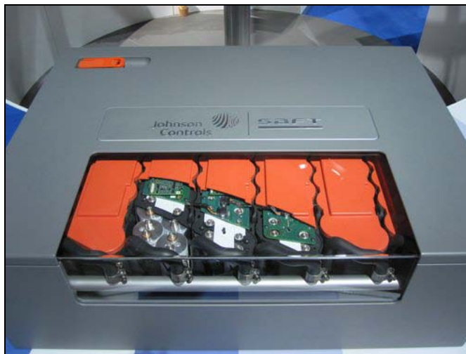
Figure 5-8: Cut-Away Demonstration Version of a NiMH EV Battery Module (Photo courtesy of NREL Photographic Information Exchange)
