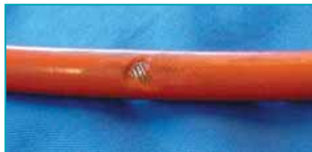
do not use damaged hose
