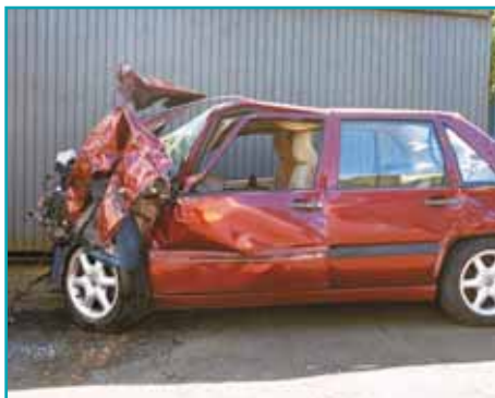
deformation due to crumple zones
