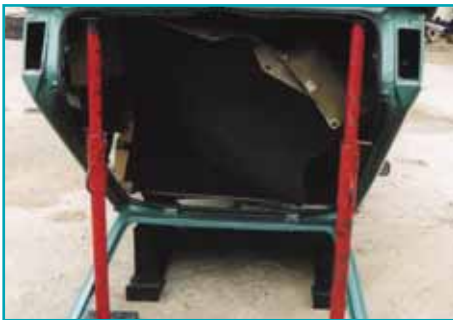
simple mechanical shoring
