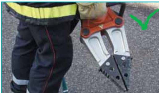
spreader carried correctly by handles
