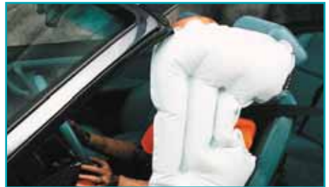
side impact chair mounted airbag
