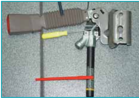
exposed seatbelt pretensioner
