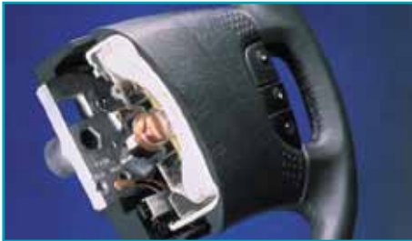
cross section front airbag undeployed
