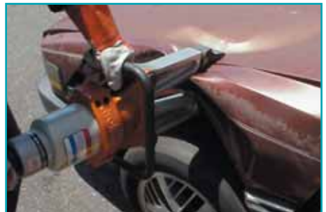
squeezing / crushing a fender
