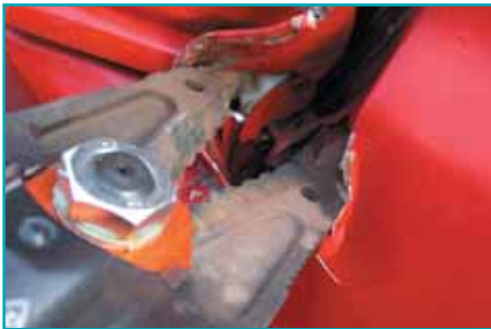
combi-tool used over locking mechanism
