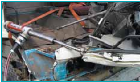
fully extended telescopic ram
