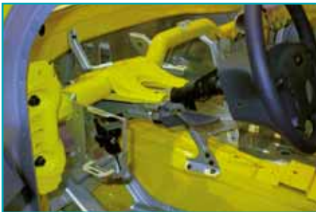
boron rod reinforcement in dashboard area may affect techniques used for dash lifts
