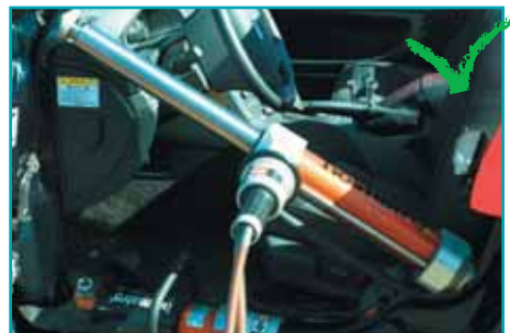
relief cut made before ramming starts
