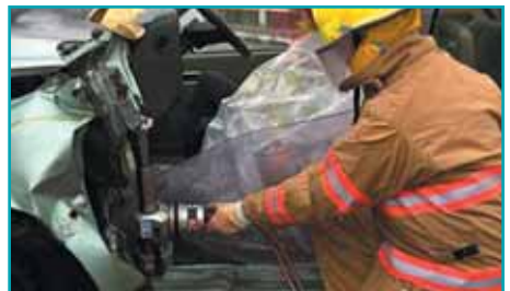
dash lift using ram
