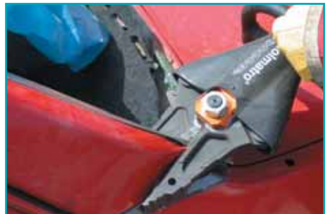
cutting a C pillar
