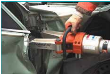
spreading a door from the vehicle
