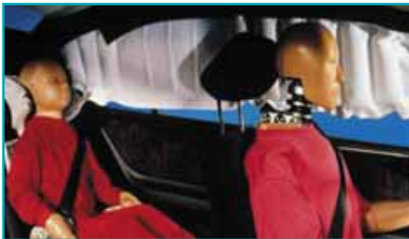
inflatable air curtain airbag
