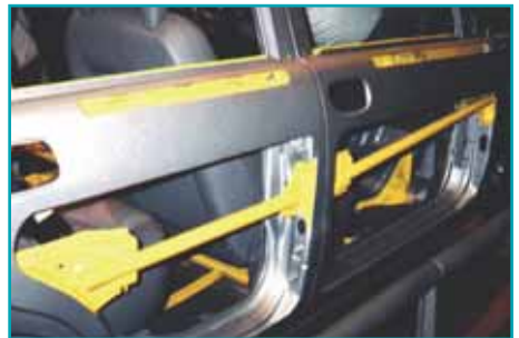
side impact reinforcement bars can lead to door removal difficulties when involved in frontal collisions
