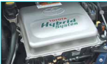
electronic drive system of Toyota "Prius"
