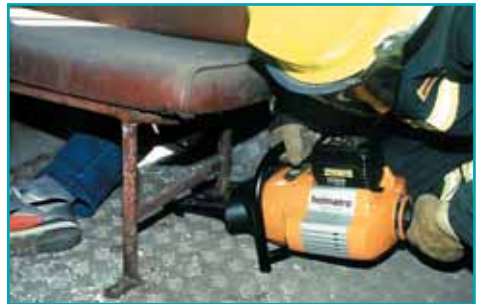
Self-contained rescue tools work well in the confined spaces of a bus.
